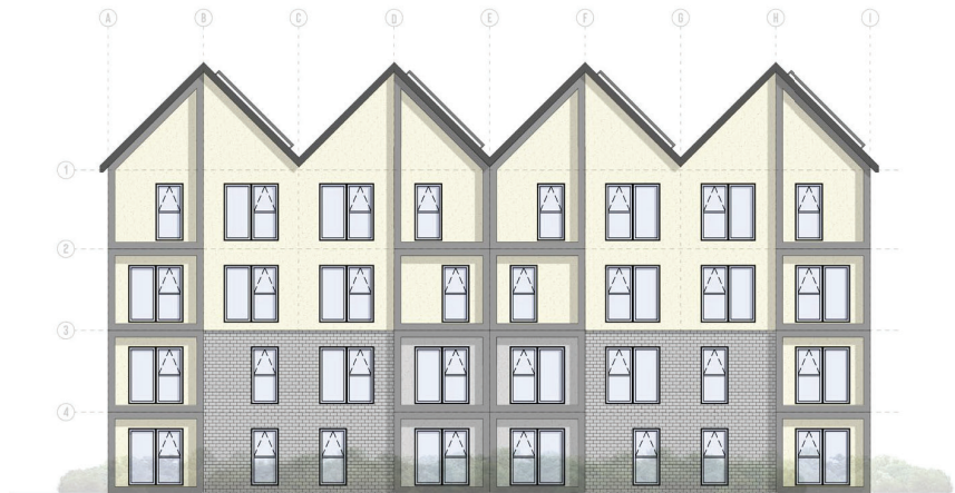
APARTMENT ELEVATION | 1:100 BRICK + RENDER
