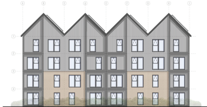
APARTMENT ELEVATION | 1:100 BRICK + METAL
